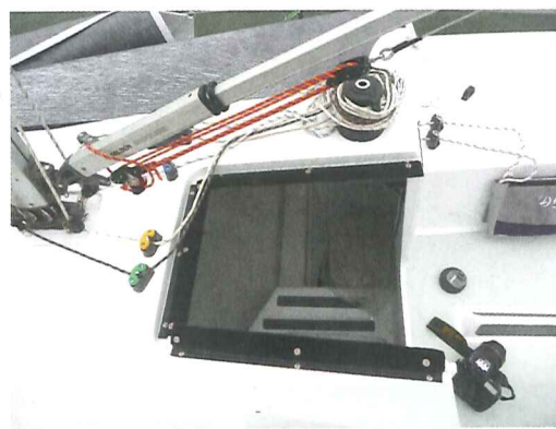
Pit area – this is simple to operate with the minimum of controls: pole in and out, kite and jib halyards, a kicker and a cunningham so no excuse to fumble
