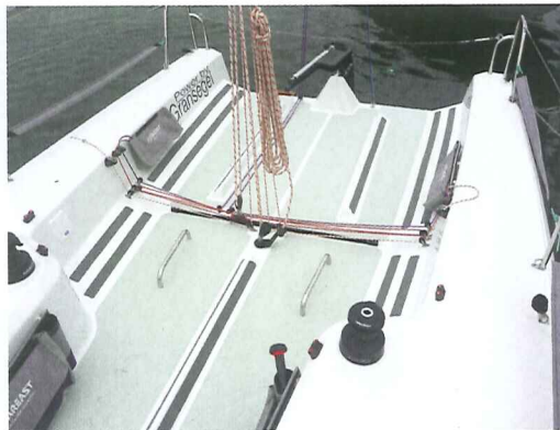
A simple, spacious cockpit can cater for five crew easily, but the narrow side decks and position of the foot braces make the cockpit less comfortable for the helmsman
