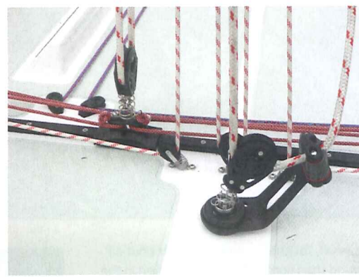
The mainsheet system comes standard with a coarse and fine-tune system with conventional traveller control line adjustments close to hand
