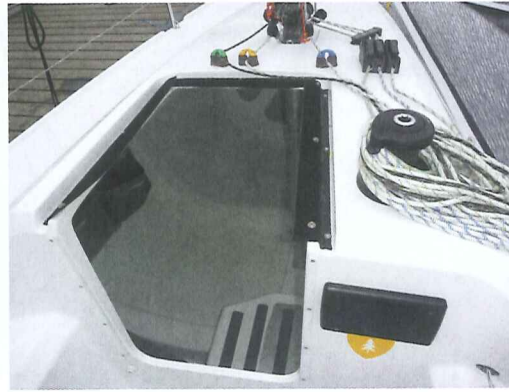
The offset companionway is very much in vogue for those who do windward-leeward racing, but the main reason is to allow you to get below when the keel is up
